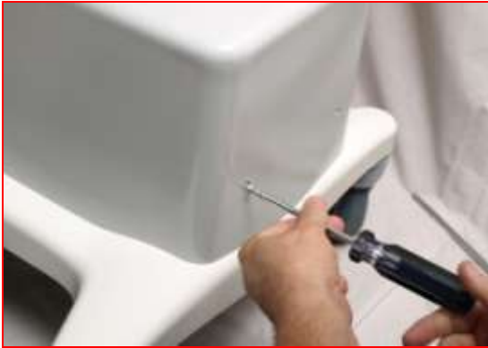
Figure 13. Removing Plastic Shroud
