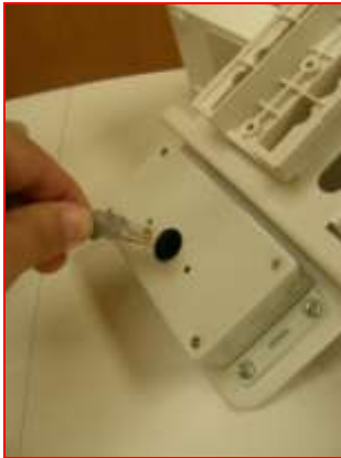
Figure 38. Plugging in RJ45 Cord
