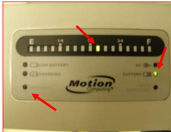
Figure 56. Checking the Battery Gauge
