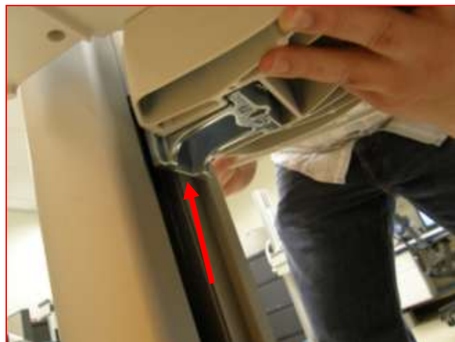
Figure 29. Sliding Large Work Surface up column
