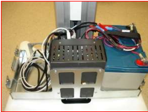
Figure 54. Securing Batteries and Cords
