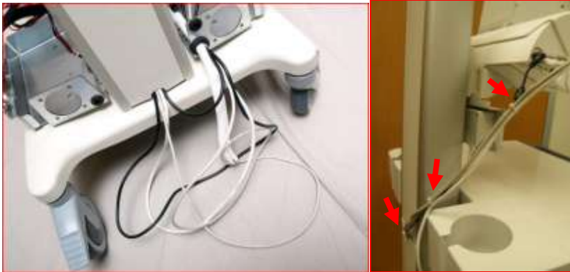
Figure 46. Pulling excess cable and securing cables
