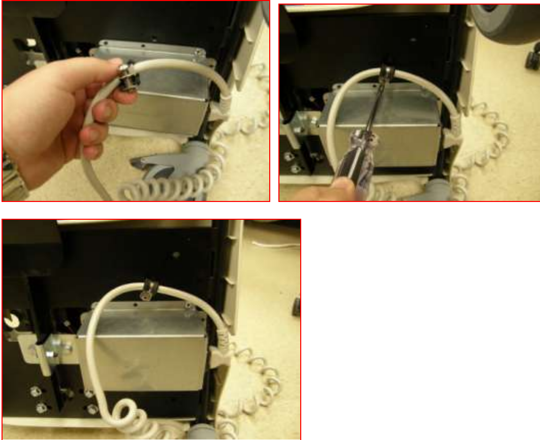
Figure 21. Attaching the Power Cord Retainer to the base
